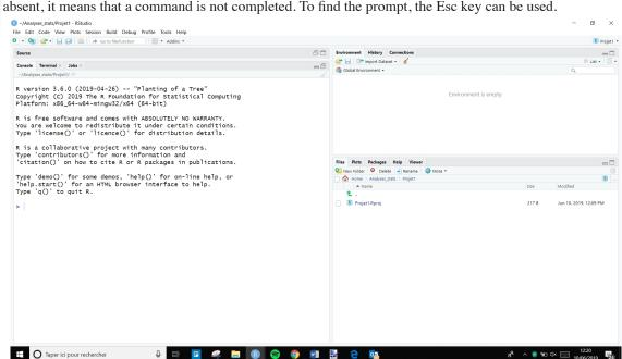
1. A command can be entered in the R console when the prompt, ie the «>» sign is present. When this sign is absent, it means that a command is not completed. To find the prompt, the Esc key can be used.
